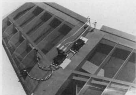
Elevator and aileron servos are both mounted in wing, mixed with Du-Bro mixer.
