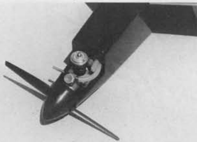
As in Whathehell, a half-A engine is used; 6-3 prop, 1-1/2-inch Goldberg spinner tops it off.
