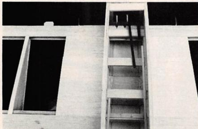
LEFT: Aileron torque rods have been added as well as spruce servo mounting strips. The spruce strip just forward of the rear fuselage sheeting is an anchor block for the radio compartment hatch. RIGHT: Wingtip showing added aileron, wingtip, and vertical grain webbing.
