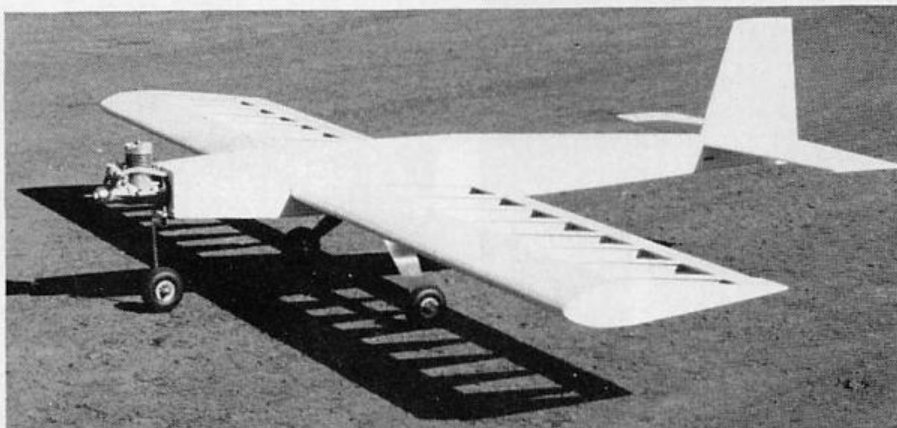
All sanded and assembled, ready for covering.
