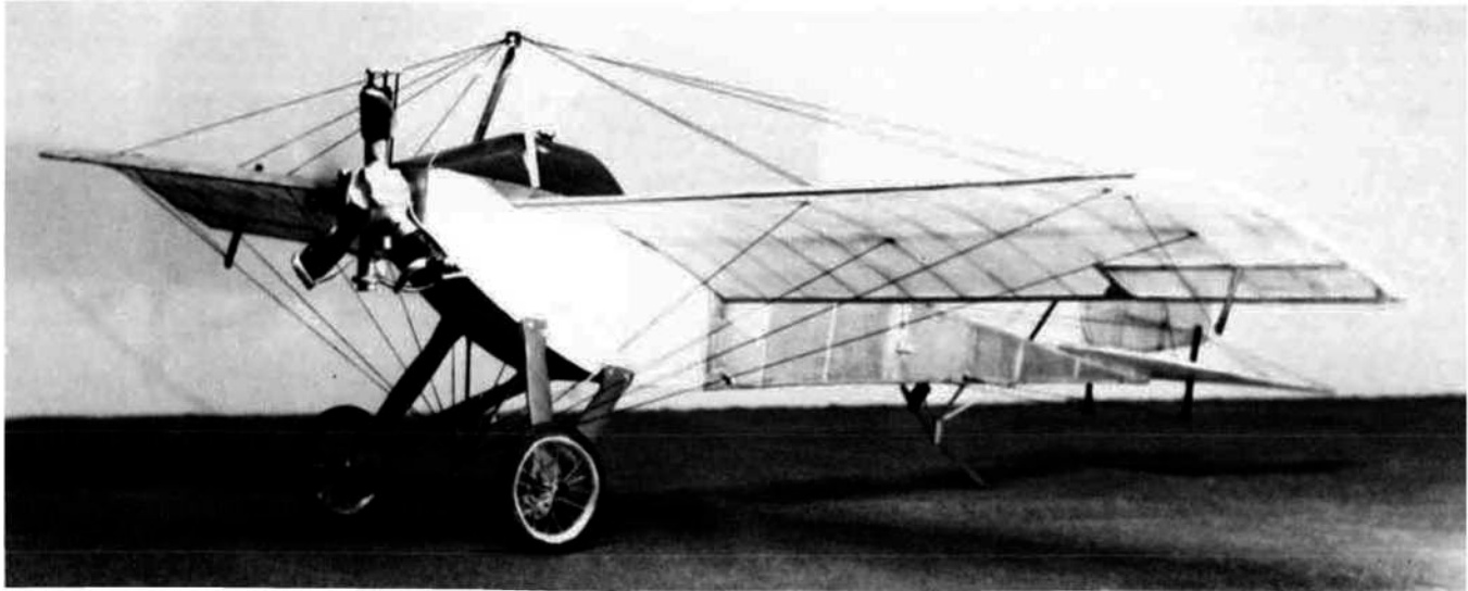
This 1913 E. A. C. Monoplane is by Bill Warner, for rubber or CO2 power. Span 19-1/2". Design won Senior at 1967 Nats for Mike Mitsch, and CO2 F/F Scale at the 1970 Flightmasters Annual (This ship. CO2 engine fits inside dummy motor.
