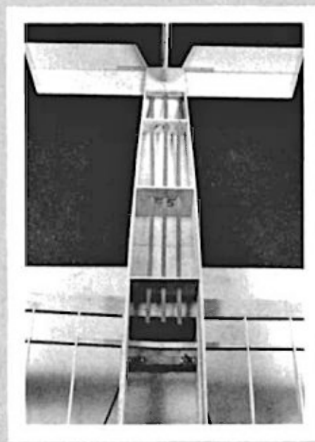
Wire landing gear assembly (above left). It's much easier to construct than it looks. Heat up your soldering iron and get going. Why are there three control rods here (above right)? Because the center rod only serves as a tube for the antenna wire, that's why! Excess antenna wire is allowed to hang out the back.
