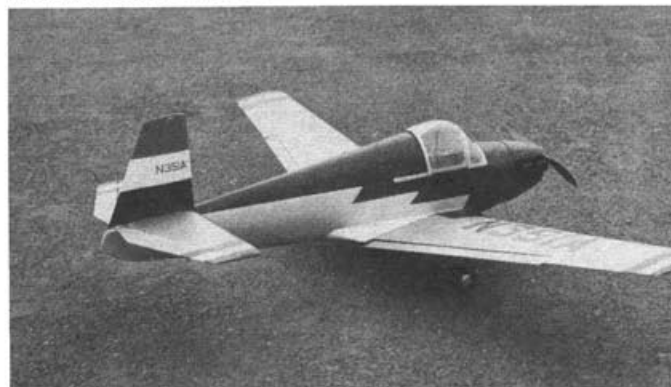
Only the usual increase in dihedral and stabilizer area departs from true scale. Tricycle gear makes take-offs thrill to watch. A prop saver.
