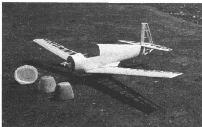
Despite sturdy construction, the little Mite weighs only 16 oz. for free flight or 21 oz. with payload. Trim, balance are same for both.
