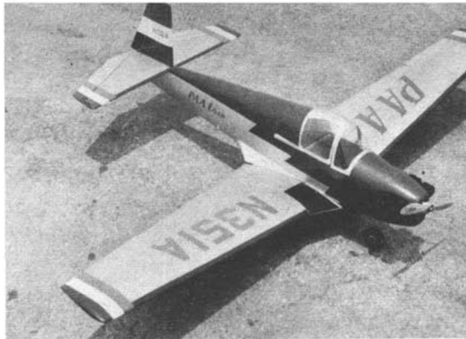
Spectacular paint scheme tops off exciting model. Canopy works. Wood is substituted for all metal surfaces and silk for fabric ones.
