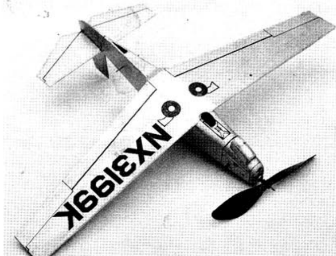
Underside view shows "retracted" gear. Dark triangle aft is access hole to rubber motor.
