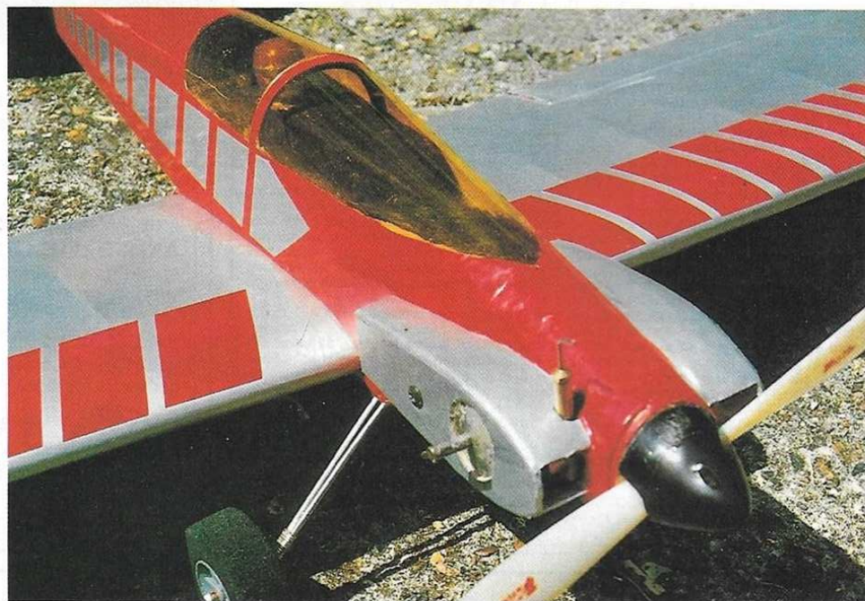
Apple-cheek cowls on prototype are pretty and simple enough to do; motor is a grand old PAW 149 with throttle.
