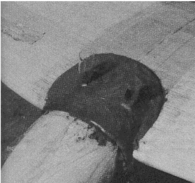
Installing bottom wing fillet, note plastic bottles for wing bolts.
