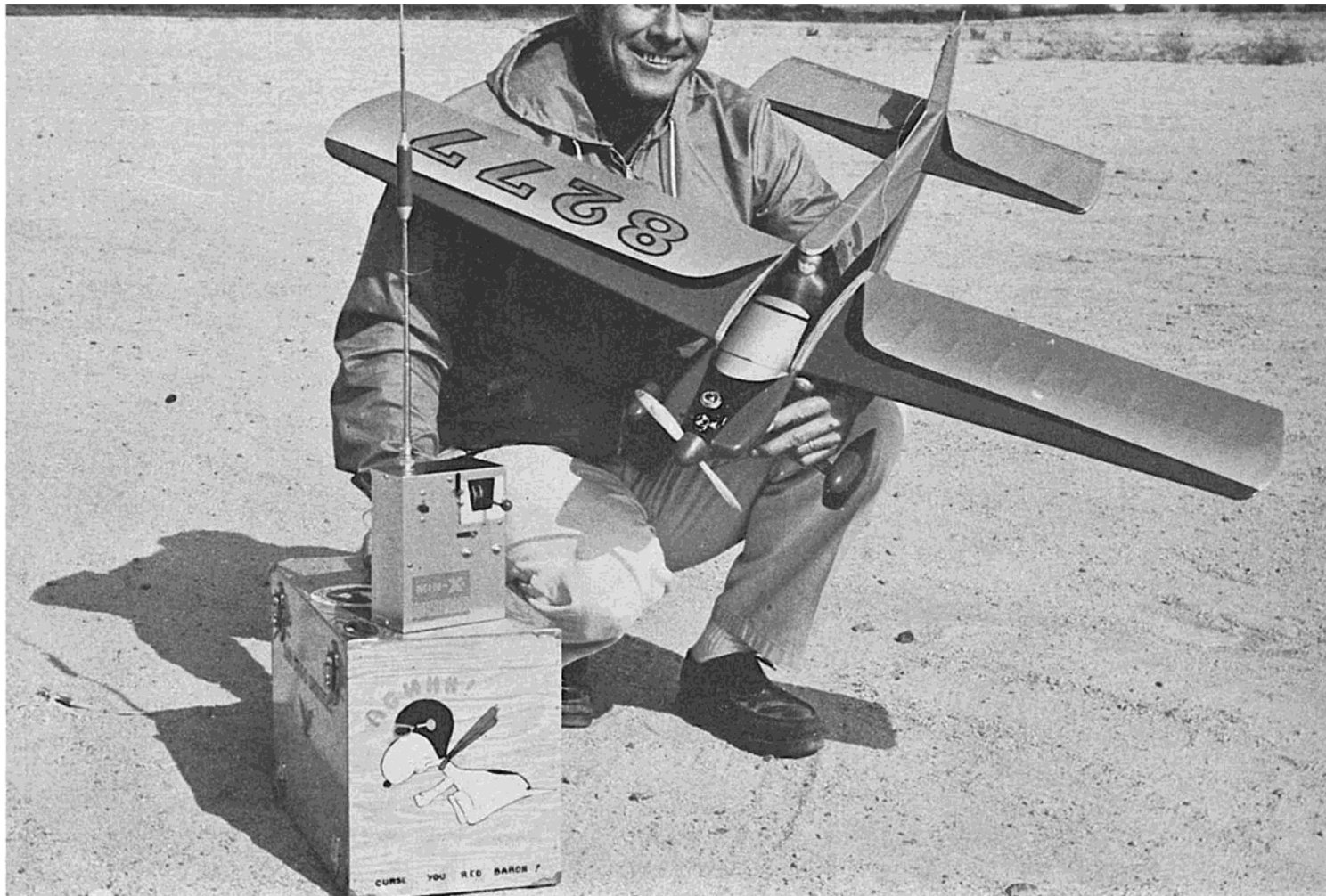
The author with his Mo-Jo prototype designed for the Midwest-RCM Air Races. Min-X 1200 Pulsemitter and Receiver, Rand LR-3 actuator, McCoy diesel. Mo-Jo is fast but easy to fly.
