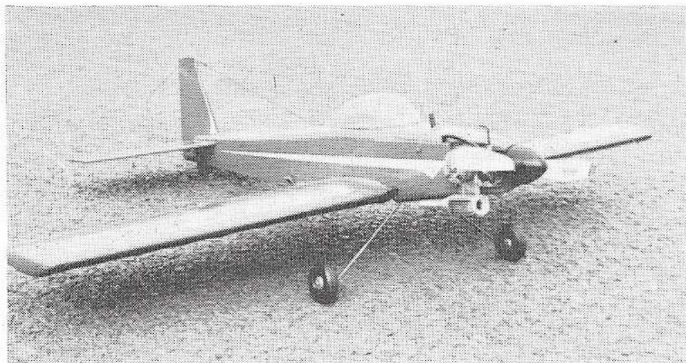
The Mite has no dihedral, which makes for simple construction, but looks a little "droopy" in this low-angle shot!
