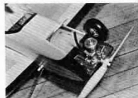
A Fox .10 nestles into front end, ample power.
