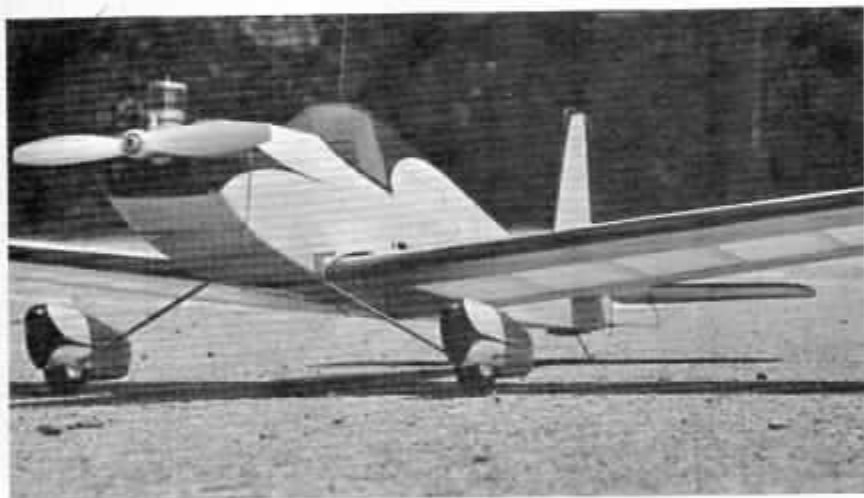
Molded pants add to appearance & reduce drag.
