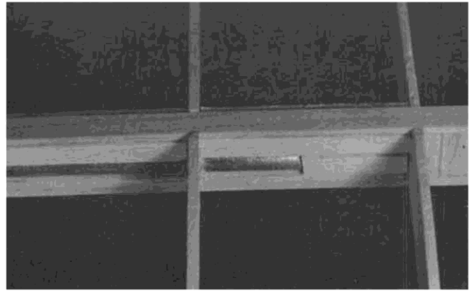
Wing tube blocked in with balsa and thoroughly epoxyed in place. Sheeting will taper load stresses.
