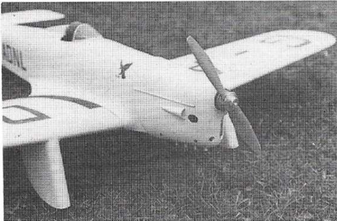
Above and bottom of page; close ups of the cowling and wheel trousers. These items are all formed easily by wrapping thin plywood around balsa formers.
