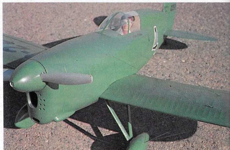
Left: Tail surfaces are solid 3/16 sheet balsa with ironed-on strips of covering material to simulate ribs. The rigging is 10-lb.-test monofilament with ends of crimped aluminum tubing. Loops of 1/32 wire are Zapped into holes through the vertical fin and stabilizer. Right: Front view shows the finished nose block in place and the little side bump. To be scale, the prop should be 14 in., but it flies with an 8-6. Cloth-wrapped balsa fairings around the landing gear wire are to scale. That is how they did it on airplanes back in the days of the Thirties.
