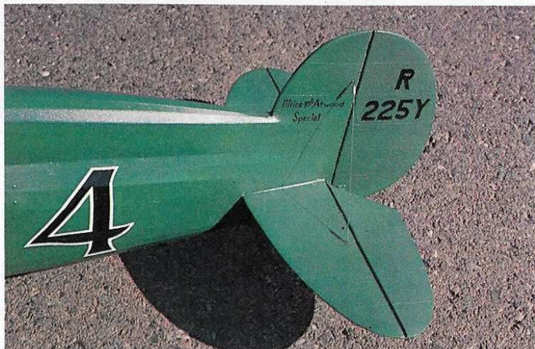
Left: Tail surfaces are solid 3/16 sheet balsa with ironed-on strips of covering material to simulate ribs. The rigging is 10-lb.-test monofilament with ends of crimped aluminum tubing. Loops of 1/32 wire are Zapped into holes through the vertical fin and stabilizer. Right: Front view shows the finished nose block in place and the little side bump. To be scale, the prop should be 14 in., but it flies with an 8-6. Cloth-wrapped balsa fairings around the landing gear wire are to scale. That is how they did it on airplanes back in the days of the Thirties.
