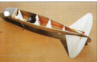
The fuselage pretty well complete (leave bottom sheering off to fix radio insulation).
