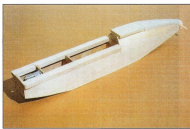
The dorsal spine has been added and the top blocks in place. Note the top keel strips.
