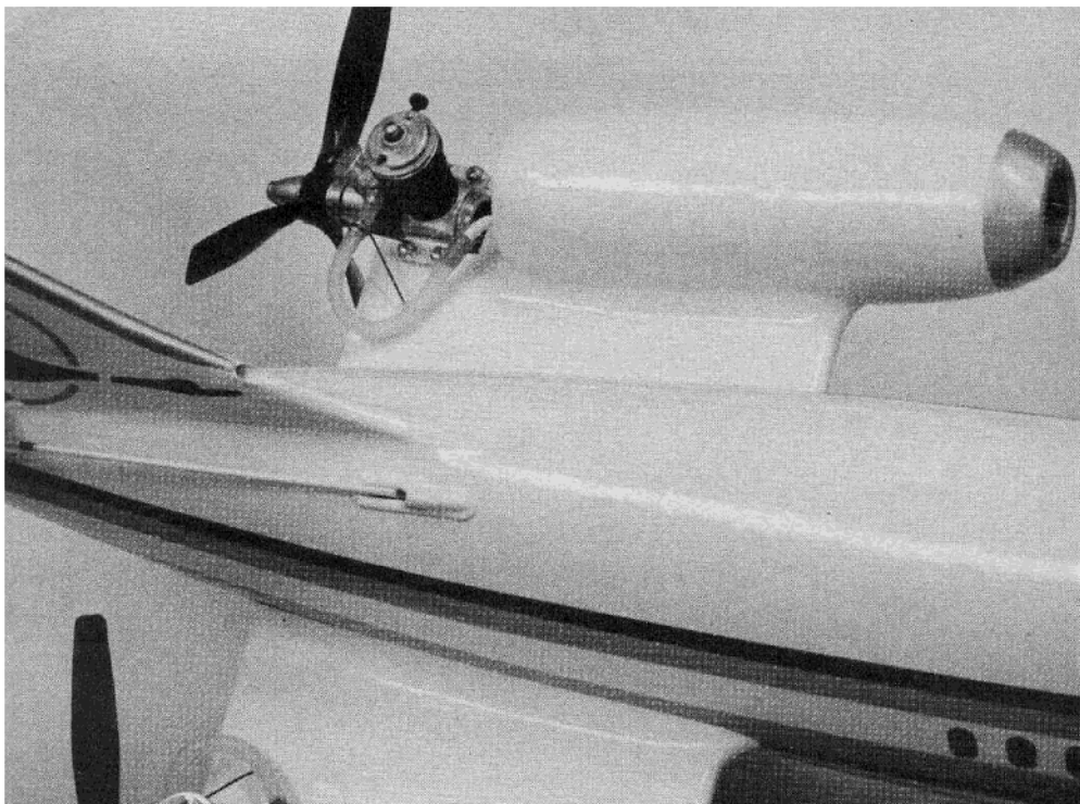
Photo #36: Engine and fuel line installation. Turn needle valves to outboard side. Note the carpet thread kill system tied to fuel line. Use a short length of brass tubing inside fuel line to avoid collapsing it with the kill line.
