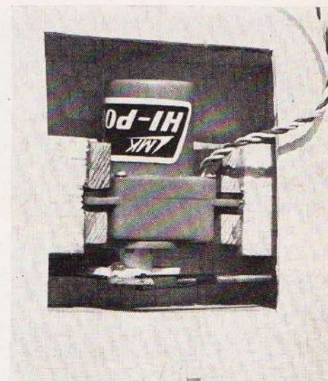
The R.M.K. retract servo which, with special Skyleader servo amplifier, has proved ideal. Skyleader make the amp. for many systems on request.
