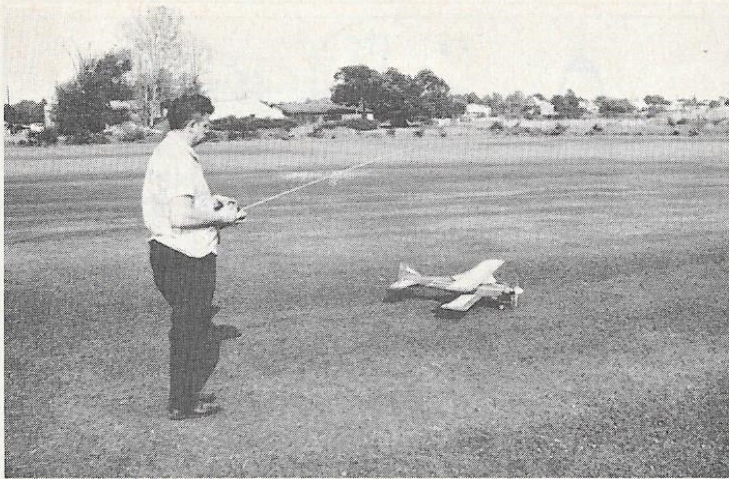
Dan demonstrates trike gear advantages. In a direct cross wind, there's no weathervaning or groundlooping. This helps if it's your first bipe.
