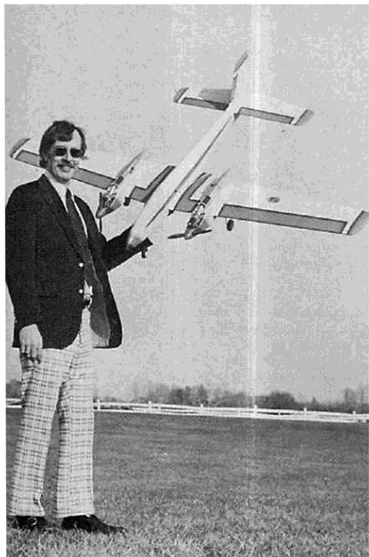
Dick and his Magnum 80 opened eyeballs at the recent WRAM's show. And it flies better than it looks. There is no shortage of power aboard, good one-engine out performance. No offset in nacelles. Top right: The K&B mill with a tuned pipe, need a pair. Electric starters make it all practical. Lower right: The new Perry carburetor provided a smoothing touch, low speed idle and reliability.
