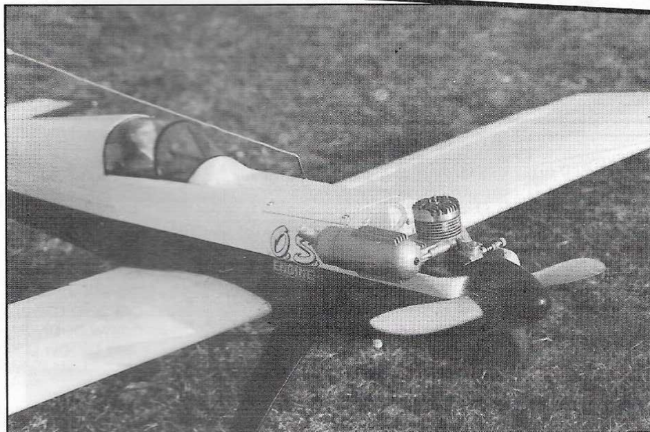
Prototype used an O.S. 40FP but engines from .35 to .60 are suitable.
