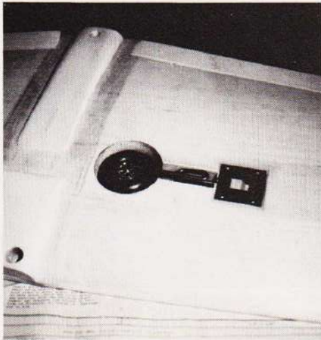
Close-up of Violett Aero main retract gear.
