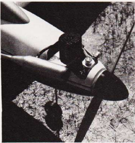
Close-up of the engine/muffler installation.
