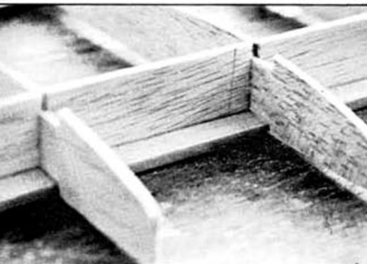
Full depth wing spar. The bottom spruce spar is glued to the vertical web before fitting the wing ribs.
