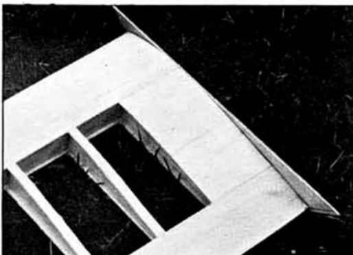
With the end plates fitted, join wings and mount on the fuselage. Shape soft balsa block to fair wing into fuselage form.
