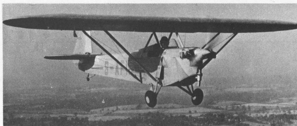
In flight, a real Luton Minor plods along. Anything from 30 to 50 hp could be used. Plans for real plane are produced by Falconar Aircraft, Edmonton, Alberta, Canada.
