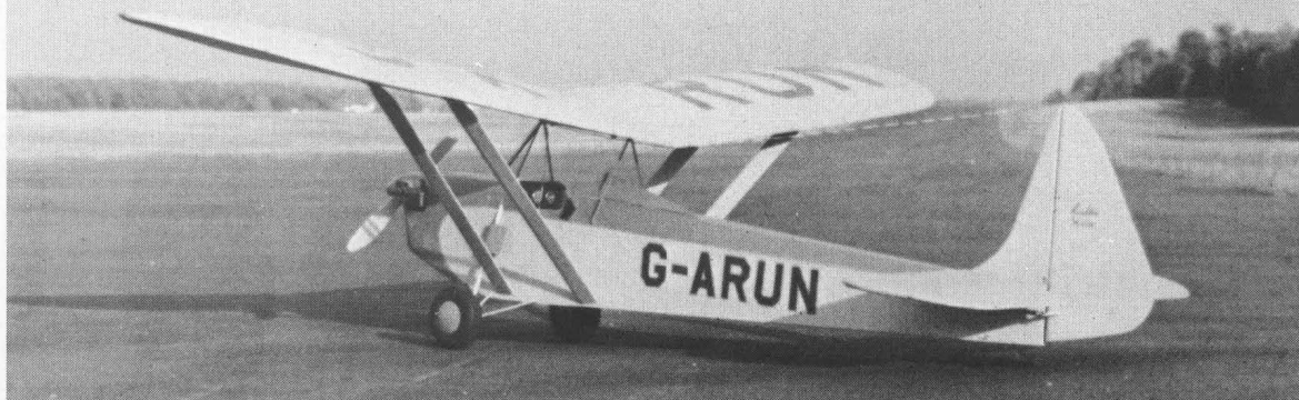
With a large rudder and plenty of dihedral, only small rudder-control movements are needed. The model has an intriguing history which began with an errant free flight near Delhi, India.
