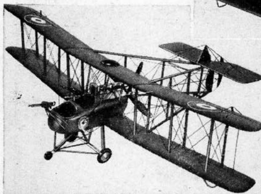
Above: No. 51—De-H-4. The first plane of its time built for 200 or better HP engines; one version using a 375 HP engine did 131 MPH, quite fast for those days. 50c
