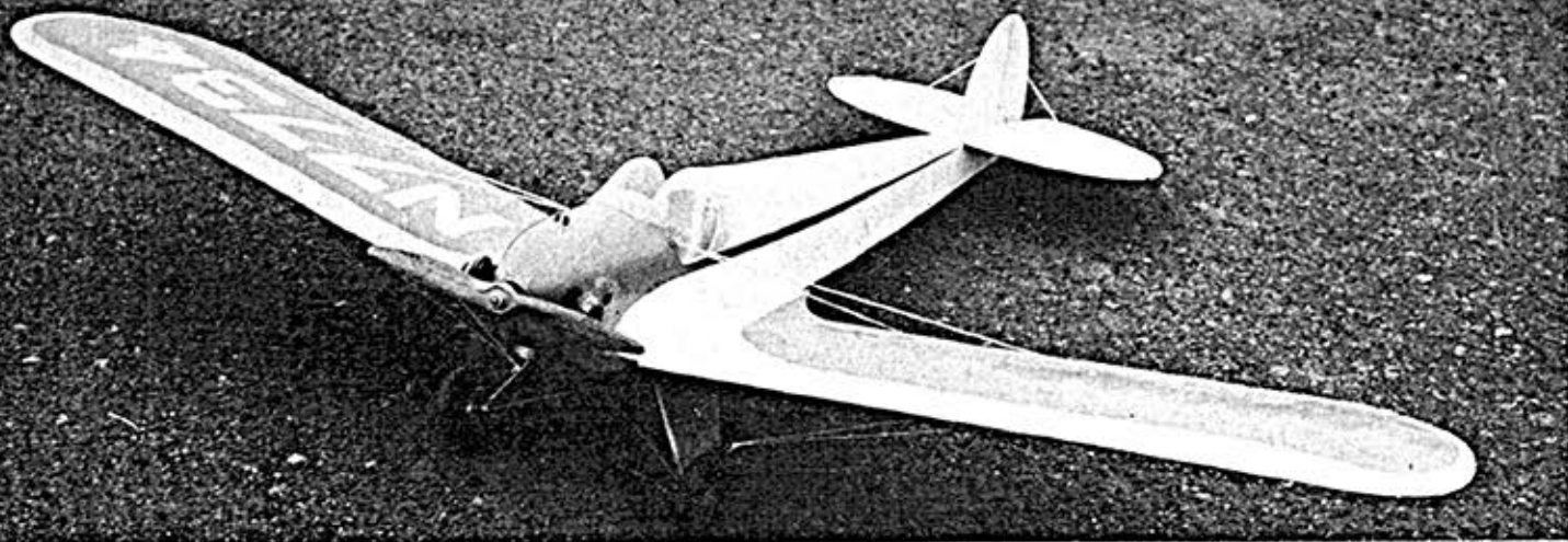
Where's the pilot? With the exception of the added dihedral this crate is authentic scale. Rubber band attachment of flying wires takes the
