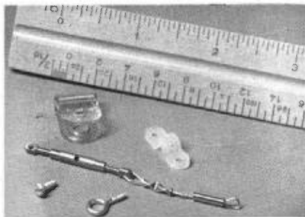
Small fittings hold plane together. Turnbuckles found at model ship suppliers.
