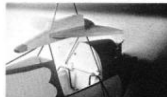
A rubber band in the fuselage provides the shock absorption. Should be fairly stiff.
