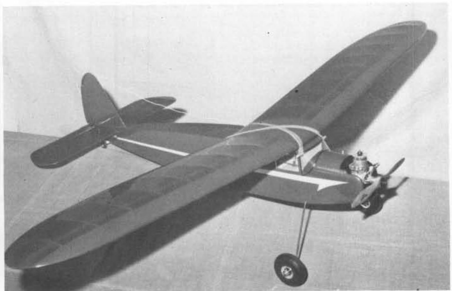
Newest 48 inch span, scaled-down old timer by Micro Models, the famous Miss America, designed by Frank Zaic. Reduced version is for light-weight 3-channel radio systems. A great trainer.
