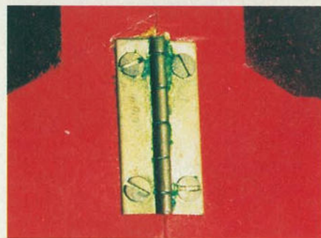
A small brass hinge joins the outer panels at the main spar.
