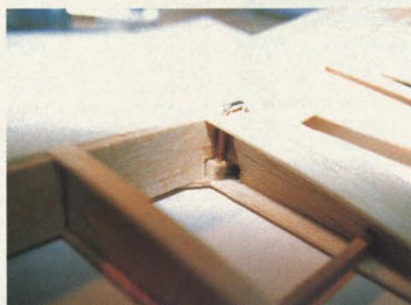
These three pictures are selected to help you around the folded wing construction. They particularly illustrate wood selection at and around the hinges.
