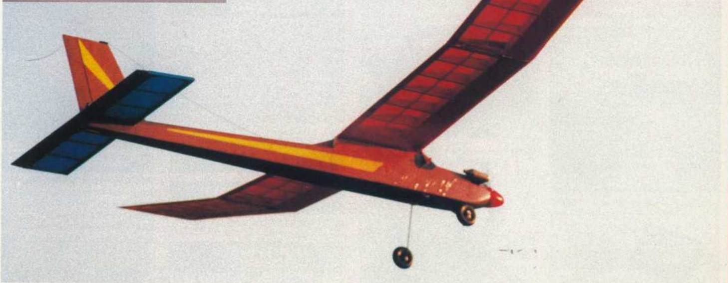
This nose-on shot shows the polyhedral wing, with fluorescent patches for visibility.
