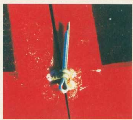
Tape is easier, but my wings are held by three 1/16" split pins, two glued through the spars into hard balsa blocks, and a third through their eyes.
