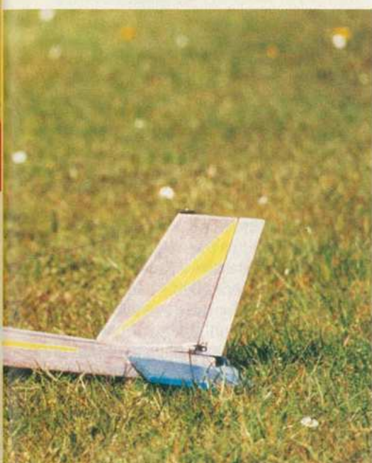
My servo installation. Note the supported snakes and minimum outer showing.
