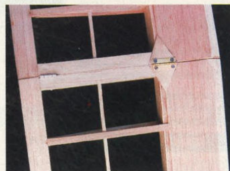
These three pictures are selected to help you around the folded wing construction. They particularly illustrate wood selection at and around the hinges.
