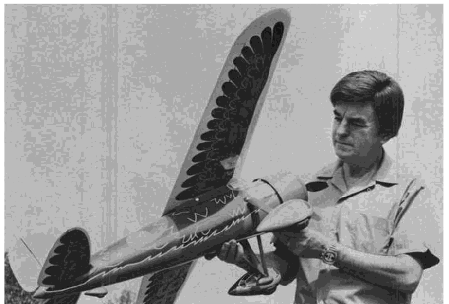
Walt justifiably admires his handiwork. Pattern on bottom side of wing and stab same as on top. Scale wheel pant blister strengthens joint to strut fairing.
