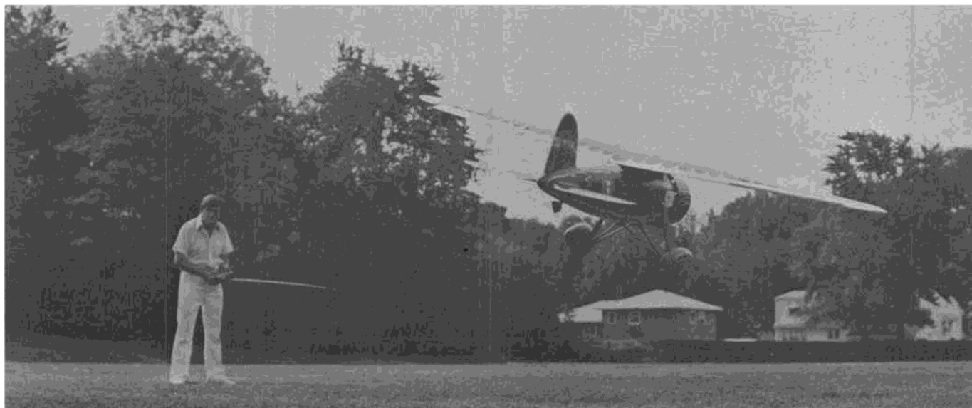
Walt brings the Vega in close for photographer, Jerry Marks. Paved runway is a must for the heavily pantted wheels. A quick removing type might be best if you have a grass flying field.
