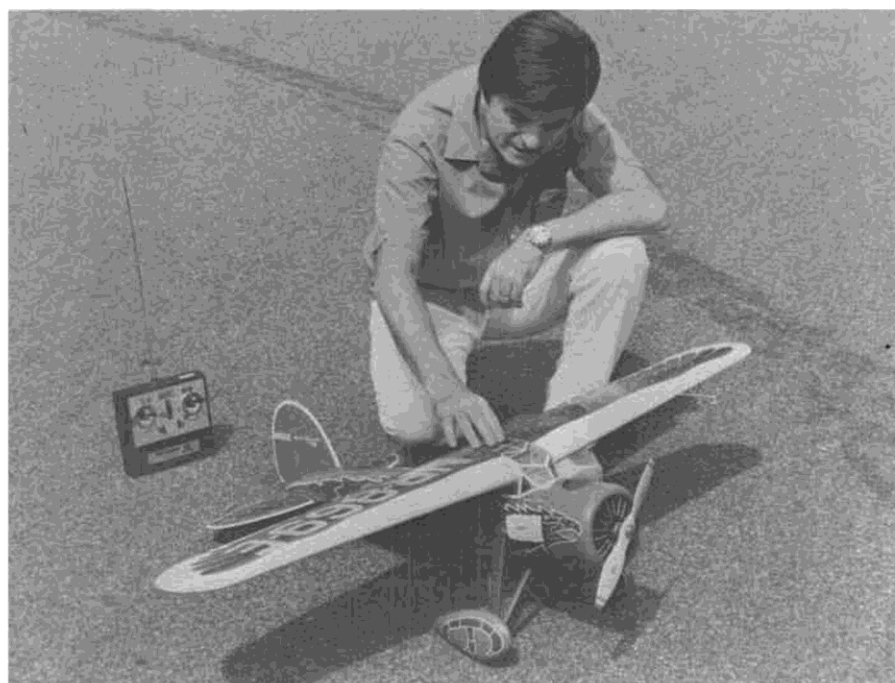
Walt opens sliding hatch on his Vega to turn on receiver switch in cockpit. Dummy radial engine is strength member of cowling, dressed up for appearance.
