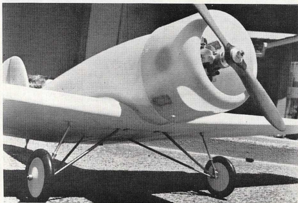
Above left: Wing center section has blocks for landing gear strut attachment and hold-down screws. There are two dihedral breaks. Above right: Rudder and elevator controls are internal and permanent. Tail cone will be epoxied in place. Left: Side mounted engine is lost in the big cowl. Muffler is housed inside entirely. Note shock strut on landing gears. Below: The symbol for Lockheed planes during the company's Detroit ownership.
