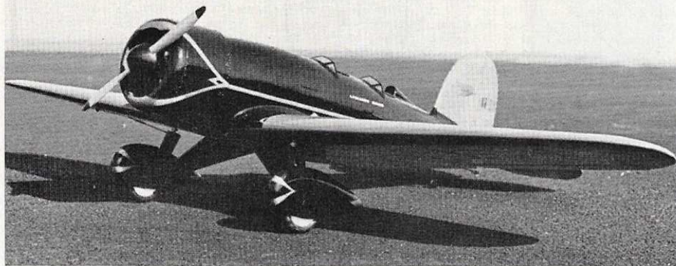
Above: Fiberglass wheel pants come with the fuselages too and are quite durable. Note plywood fill-in between inner landing gear struts. Right: Cowl alignment jig taped in place. Below: Fiberglass cowl has tabs epoxied inside for attachment to firewall.
