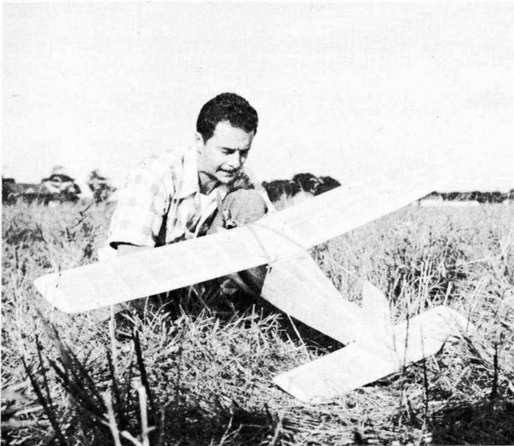
Single-spar wing is knock-off in crash, ties on with rubber looped over two rear, one front, dowels. Stabilizer detachable, ties in place under fuselage. Team racer gear.
