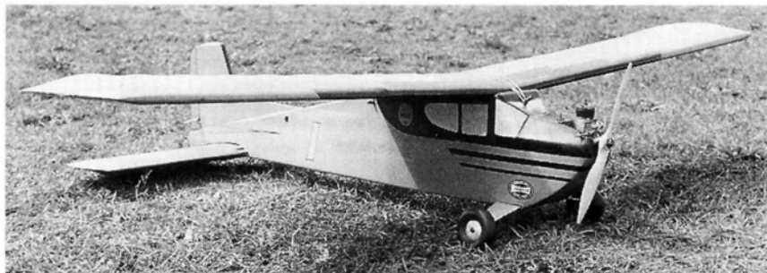
The original Live Wire Senior, powered by a K&B .19 engine and guided by a C-S 465 radio. It logged 124 flights before its escapement rudder froze during winter flying.
