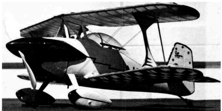
When it comes to scale detailing, you can't do better than to own the plane you're modeling! Note the similarity in this photo to the one above. Note CO 2 fill nozzle under fuselage.
