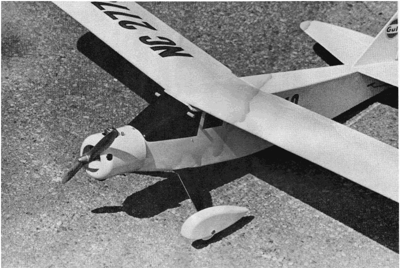
Simple sheet balsa "box" construction and ABS plastic pharmacist's pill bottle cowl makes construction a snap.
