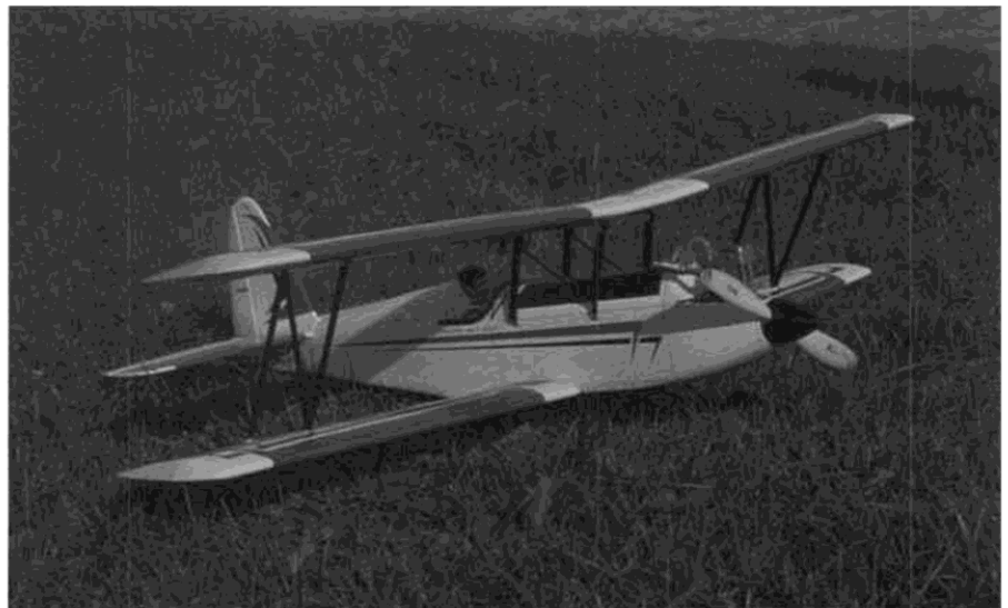
First flights were made with an O.S. 40 four-stroke, but the engine lacked the punch needed for aerobatics, so a Surpass .48 was installed, which greatly improved the plane's performance.
