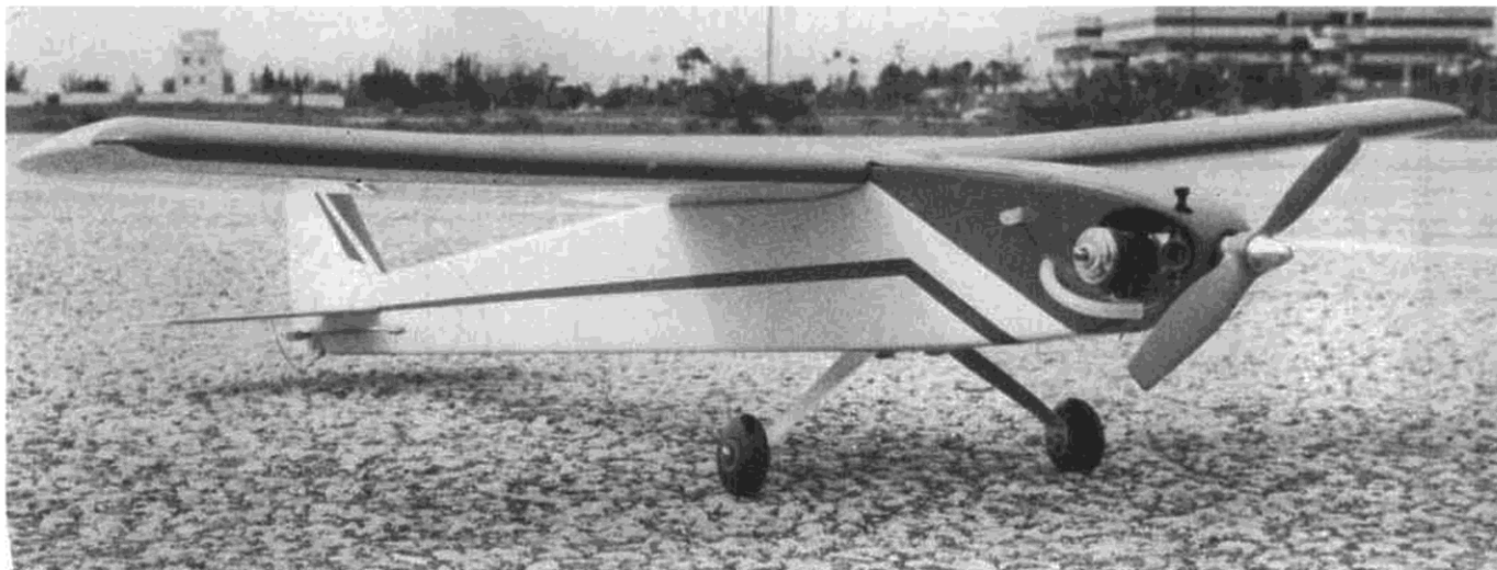
How to make a Cox .049/.051 look big . . . put it in a small airplane!. The fuel line looks like a smile on "Little Bomb."
