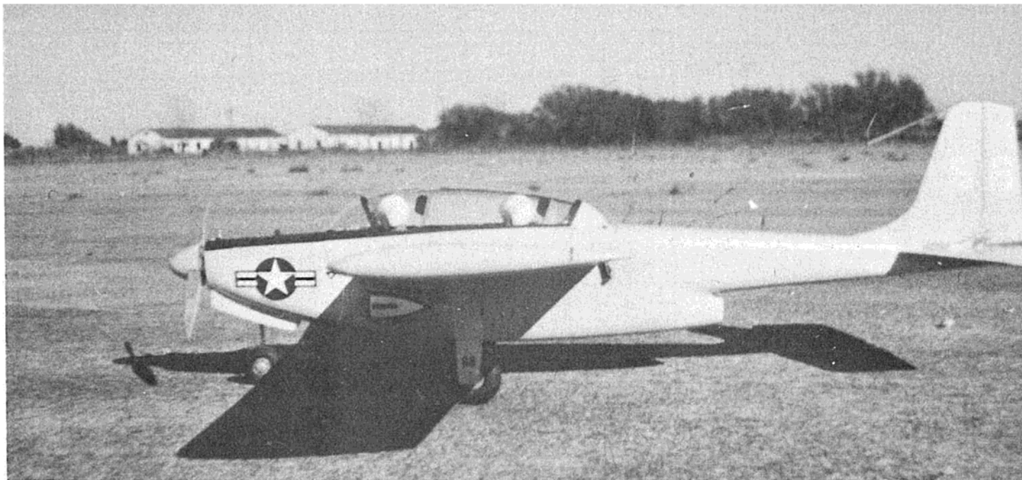
Full side view of the Li'l Pinto evidences realism achieved by use of noes wheel door, wing mounted main gear, and jet exhaust.
