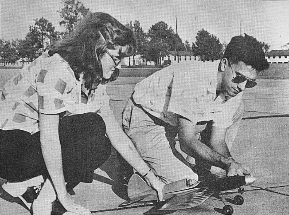
Just before take-off, the author adjusts the needle valve on Torp .15. Spinner looks good.
