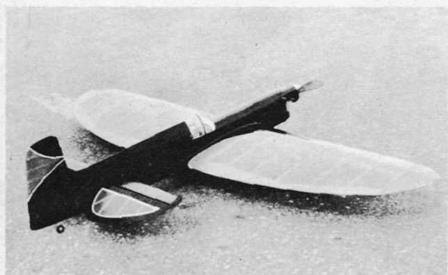
Profile distinctive for a stunt design. Long fuselage, inverted engine, cause the ship to sit almost horizontal to ground. Helps take-offs.
