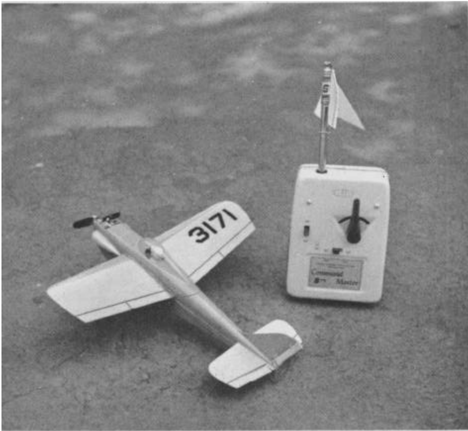
A little bit smaller and Mac could use his Sterling Command Master for a carrying case. Mac got ten or more flights of 2-3 minutes each from Eveready #S76 silver-oxide cells substituted for the German carbon-zinc cells.
