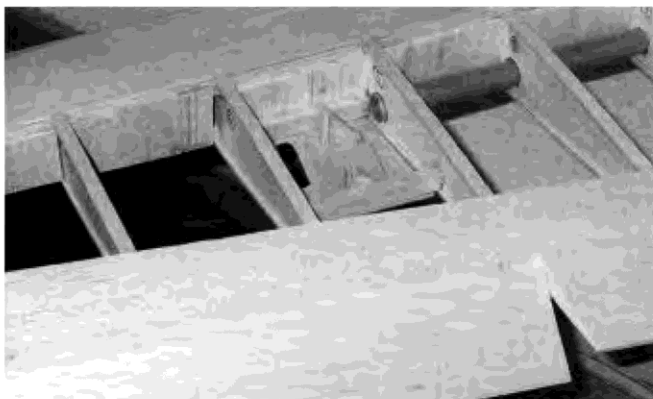
Wing is initially framed upside down. Using a long metal ruler ( above left ) helps to check for straightness of the leading edge. Building of the removable cockpit can be completed after the wing is solidly mounted ( above right ). 1/8-inch balsa
