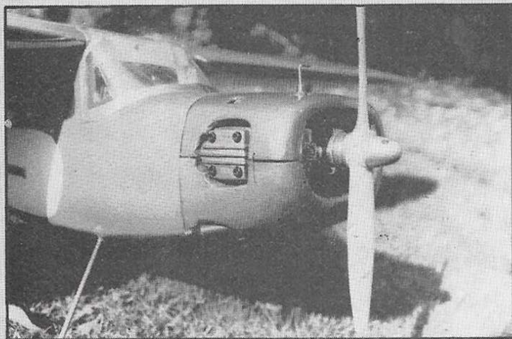
The Lady Eowyn was designed around the HP VT-21 and the width of the cowling suits this engine exactly.
