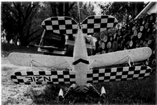
Checkers anyone? Red and white color scheme leaves no doubt as to the plane's attitude in flight. Tail brace is important with big engine.
