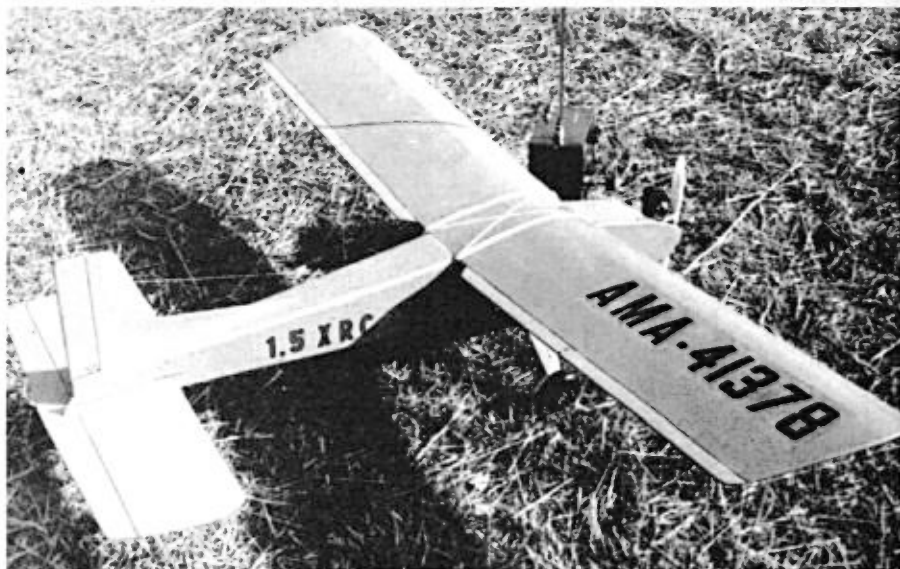
Original Klutz Bug with straight-up vertical rudder. This version used a McCoy .35 R/C en-
