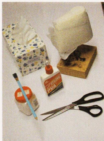
Covering cowling plug with tissue to smooth the finish
