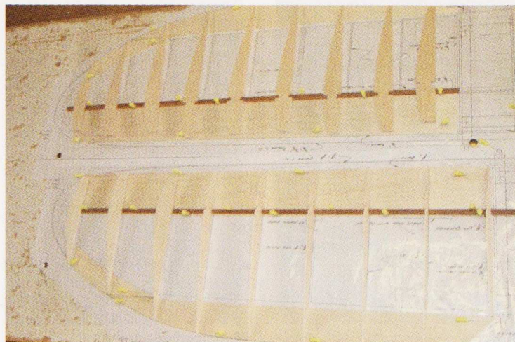
Laying up wing panels
