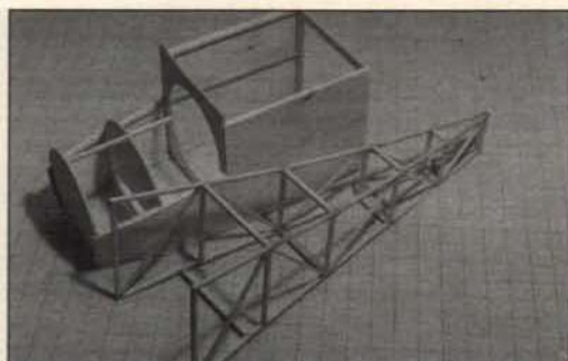
■ LEFT: Wing construction is pretty basic. Note that the upper main spar is positioned below the surface and runs through a rectangular hole in each full rib. Spars are spruce and the wing struts are functional, but you still might want to add shear webs between the spars for extra strength. ■ CENTER: Fuselage is built in two sections, front and back, then spliced together. ■ RIGHT: Rather than mess with clear plastic windows, the author quite sensibly chose to go with painted windows (light blue MonoKote, actually) and a stronger, easier all-balsa cabin. Seen here is the 1/16 balsa "windshield" after being glued in place.
