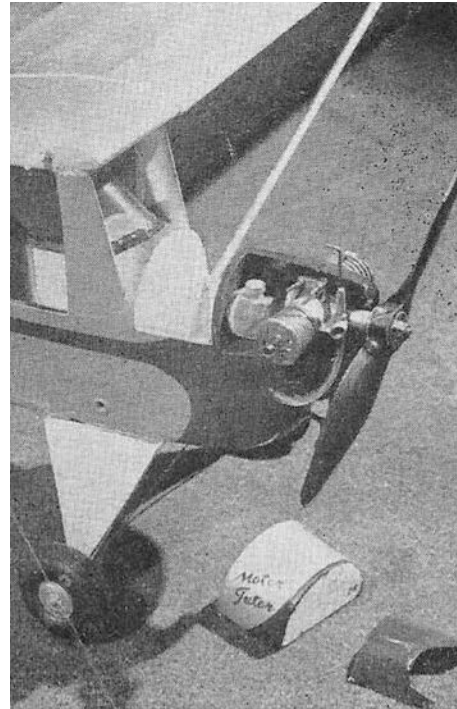
Photo shows engine installation.
