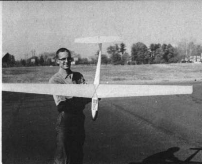
Do you have to drive miles to get to a field where engines are tolerated? Here is the answer. Dave shows easily built, high A/R sheet wing.
