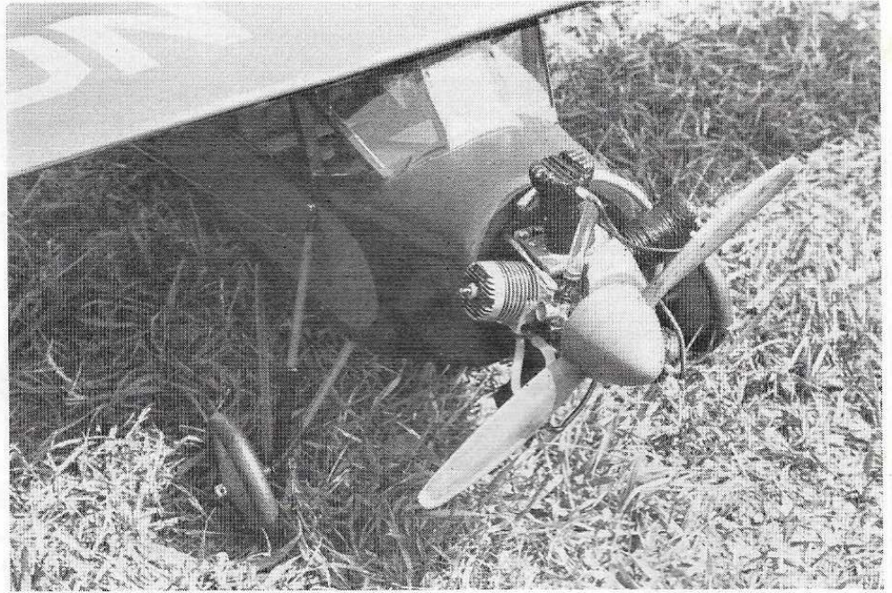
A good .35 will fly the Kari-Keen very nicely and can be incorporated in a dummy radial engine block. Right thrust is required and can be built into the firewall. Also, make sure plane balances on the C.G. shown.
