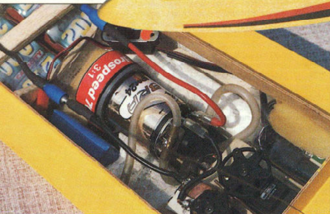
Below: Current installation which uses a water-cooled motor and simple servo operated on/off switch.
